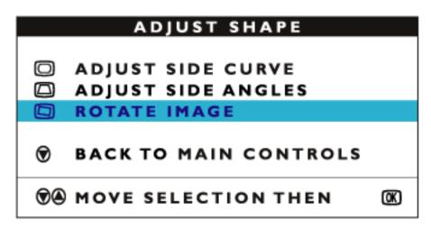
5) Press the **log** button. The ROTATE IMAGE window appears. ROTATE should be highlighted.
